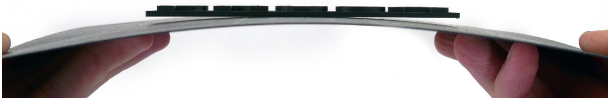
Pict. 14 - Removing the model from the PEI print surface by bending the steel sheet.
