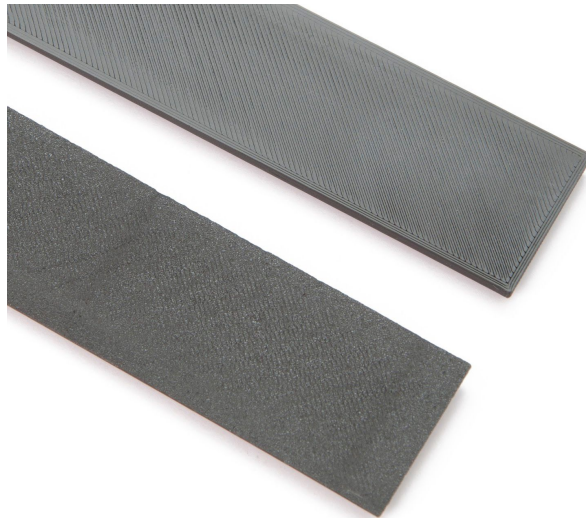
Pict. 7 - Smooth PEI sheet (top) vs textured powder coated PEI (bottom) effect on first layer
